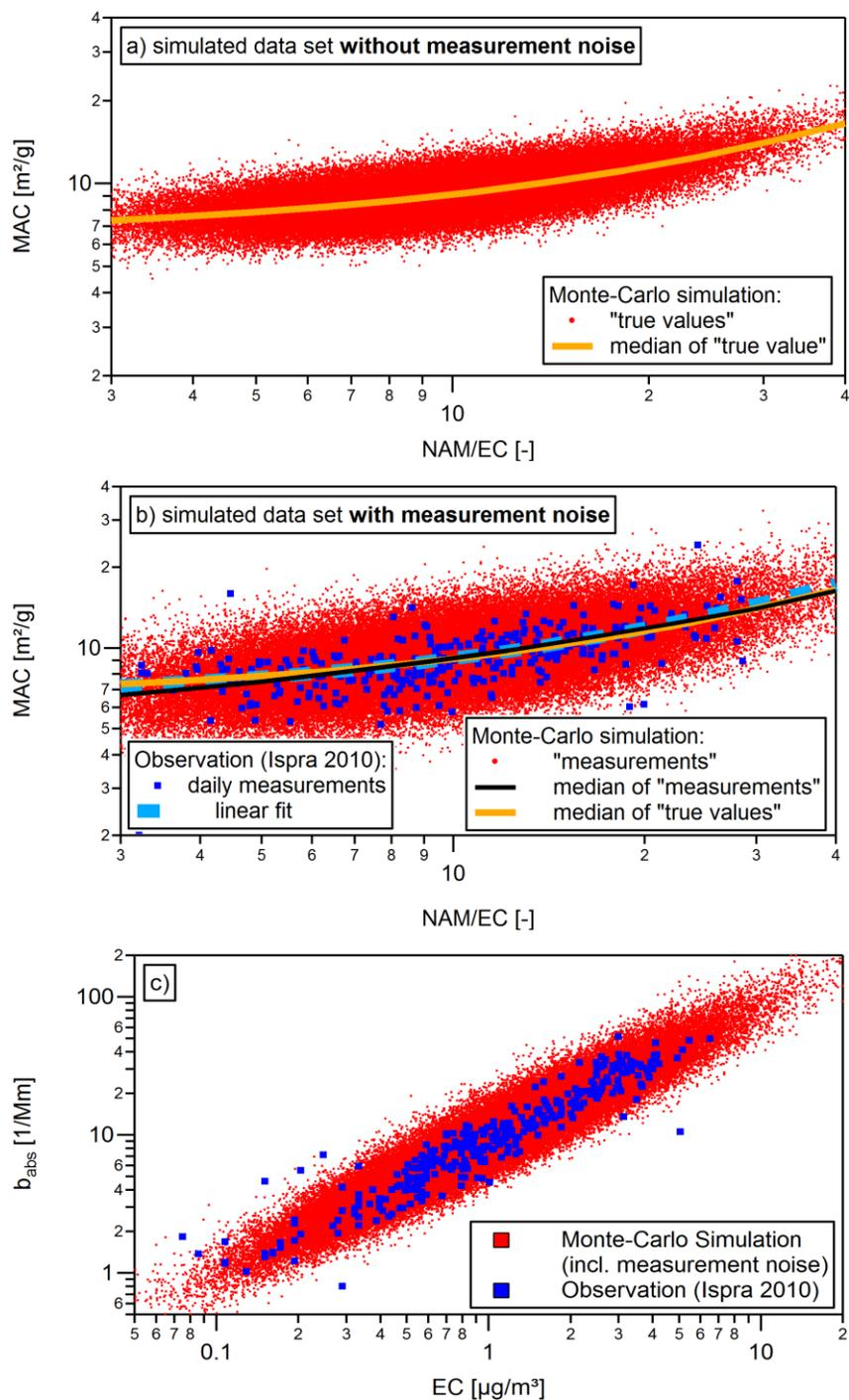
**Figure S3.** Monte-Carlo simulation of the effects of measurement noise for case 1. (a) MAC as a function of NAM to EC ratio for prescribed "true values" without random measurement noise and (b) simulated measurement with random noise and (c) absorption coefficient as a function of EC mass concentration.
