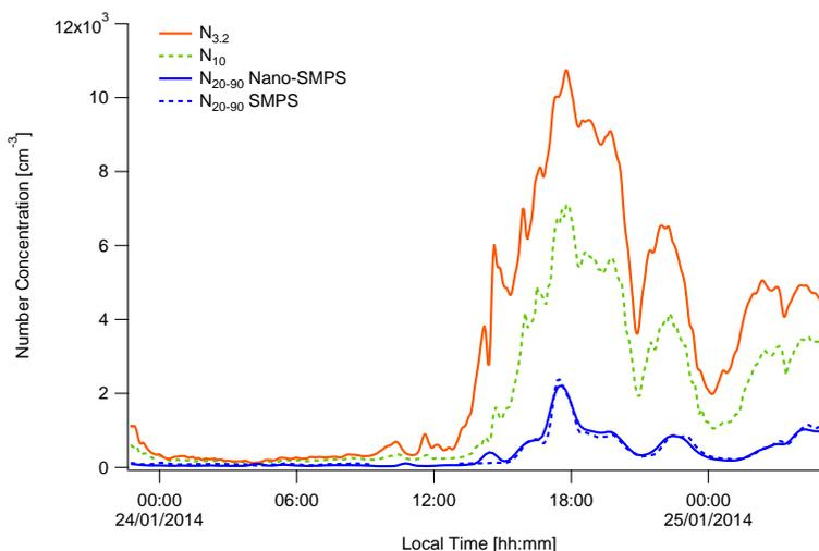
Figure S1: Comparison of total number concentration during nucleation event measured with nano-SMPS  $N_{20-90}$ , SMPS  $N_{20-90}$ , CPC 3772 ( $N_{10}$ ) and CPC 3776 ( $N_{3,2}$ ). After diffusion loss, charging efficiency and CPC detection efficiency correction there is excellent agreement between SMPS and nano-SMPS.
