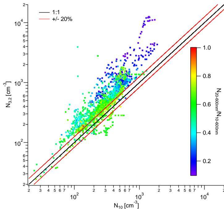
Figure S2: Detailed comparison of CPC 3772 ( $N_{10}$ ) and CPC 3776 ( $N_{3.2}$ ). Due to the different cut-off efficiencies, we expect that  $N_{3.2}$  is always larger than  $N_{10}$ , as the aerosol number size distribution is generally dominated by particles in the Aitken and nucleation mode (see Figure S3). At times when the cut-off difference is of minor relevance, the two CPCs are within  $\pm 20\%$ .
