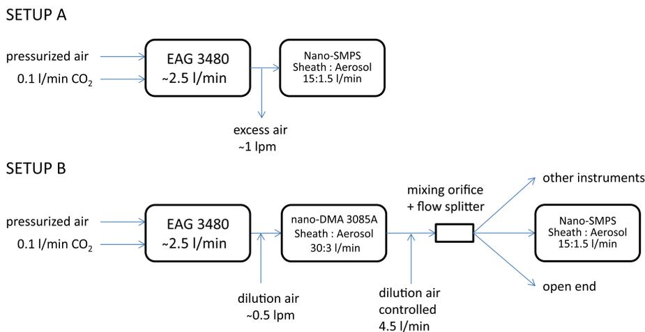
**Fig. 2.** Schematic of the characterization experiment showing two different testing setups. Setup A was used to acquire size distributions of different electrospayed solutions. Setup B was used to generate monodisperse distribution which were then subsequently measured with the Nano-SMPS. For this a second DMA was needed to select particles of a certain size beforehand.
