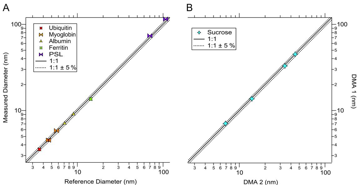
**Fig. 4.** SMPS sizing experiment. The left plot shows the observed  $D_g$  in comparison to the reference values from literature or manufacturer data. The standard deviation was less than 1% and is, therefore, not plotted. The right plot shows the comparison of SMPS 1 and SMPS 2 to verify the two DMAs against each other. Also here the standard deviation was less than 1% and, thus, not plotted.
