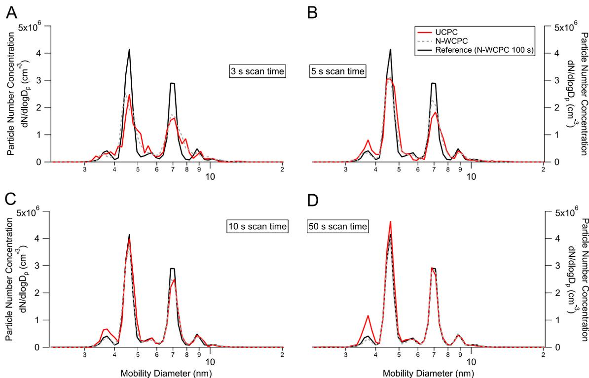
**Fig. 8.** (Color available online) Comparison of the N-WCPC and the UCPC as detectors in the Nano-SMPS. The performance using different scan times of the N-WCPC and UCPC are compared to a reference scan of 100 s performed by the N-WCPC. (A) corresponds to 3 s, (B) to 5 s, (C) to 10 s and (D) to 50 s.
