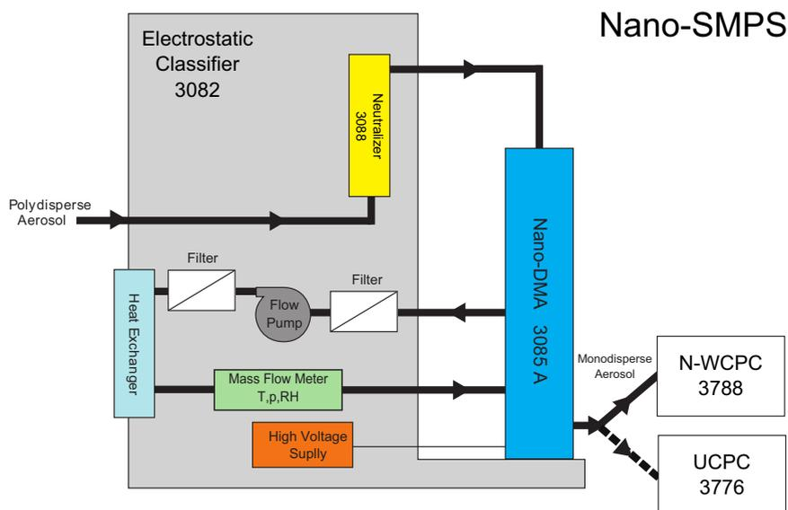
**Fig. 1.** Nano-SMPS. Operation schematic of the new Electrostatic Classifier (EC, TSI 3082), with the new sheath flow pump for increased flow rate and the precision dynamic, the soft-X-ray bipolar aerosol neutralizer (TSI 3088), Nano-DMA 3085A and CPC. The water-based N-WCPC was mainly used in this study, in some cases (when stated explicitly) a UCPC 3776 was used.
