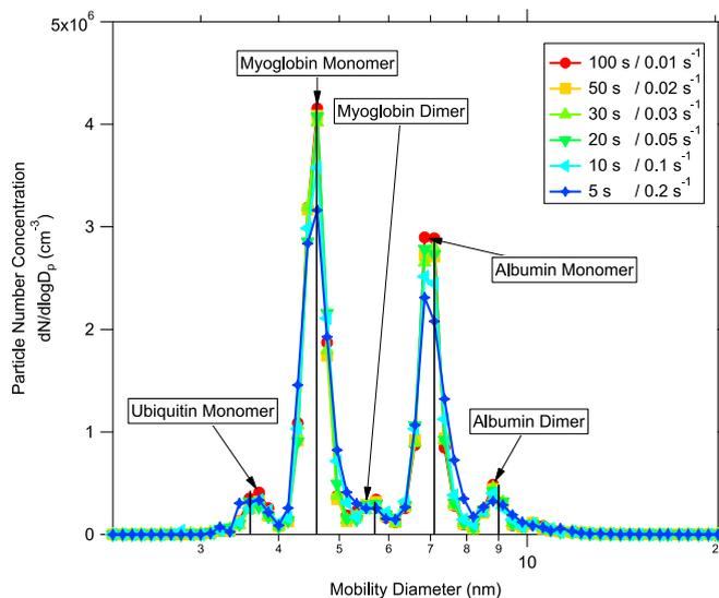
**Fig. 6.** Fast scanning multi-peak solution of the proteins ubiquitin, myoglobin and albumin. Different scan times were tested to investigate their influence on sizing and resolution. The observed peaks correspond to: (1) ubiquitin monomer, (2) myoglobin monomer, (3) myoglobin dimer, (4) albumin monomer and (5) albumin dimer.
