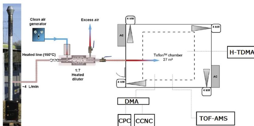
**Fig. 1.** A sketch of the setup of the wood burning measurements, including the burner, smog chamber and instruments that were measuring. Adapted from Heringa et al. (2011).
