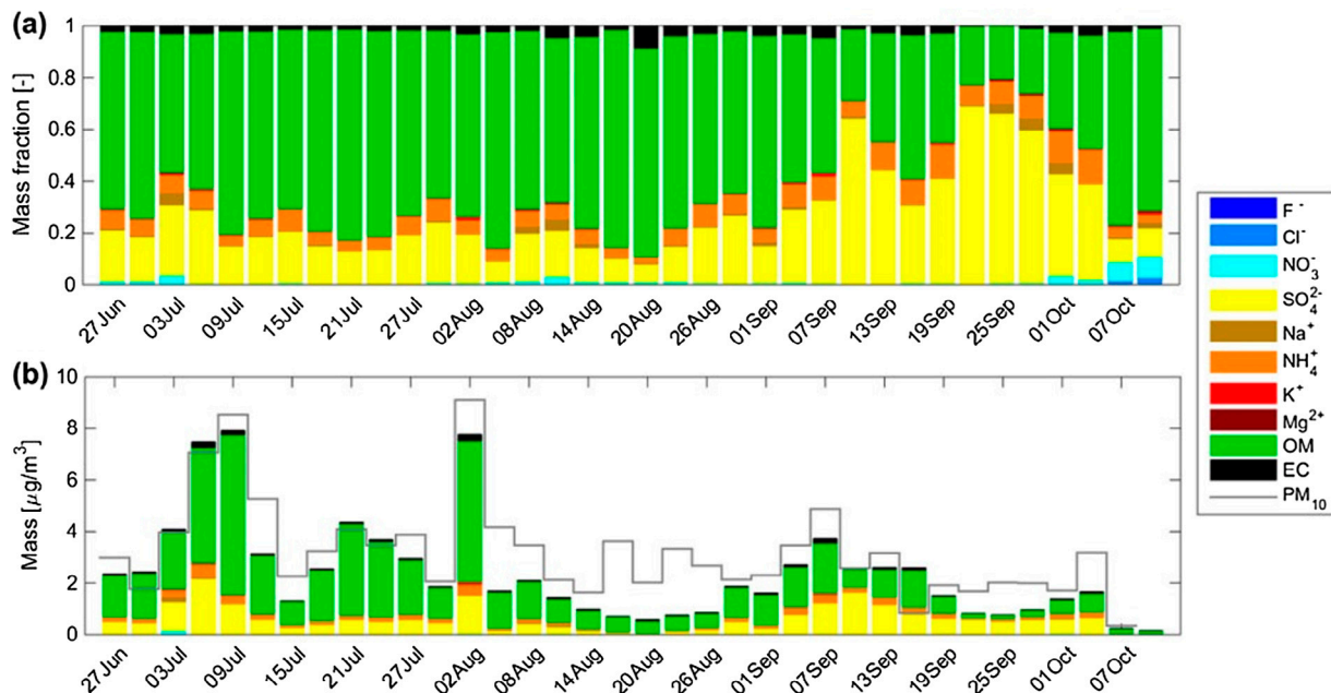
Fig. 3. Time series of (a) the 72 h mean mass fractions of the total analysed mass and (b) the 72 h mean absolute concentrations of the measured aerosol components. The grey line in (b) shows the estimated total aerosol mass for \text{PM}_{10} derived from particle size measurements with the assumptions that all particles were spherical and that they had a mean aerosol density of 1.5 \text{ g cm}^{-3} .
